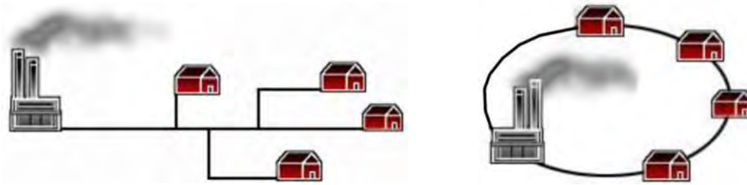
Image 4 - Radial (left) and Loop (right) network systems
